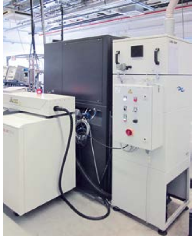
Laser welding system with integrated fume extraction system
